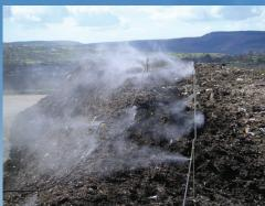
A portable, highly effective, high-pressure, multi-nozzle, finely atomised mist delivery system for short term dust suppression and/or odour control.
